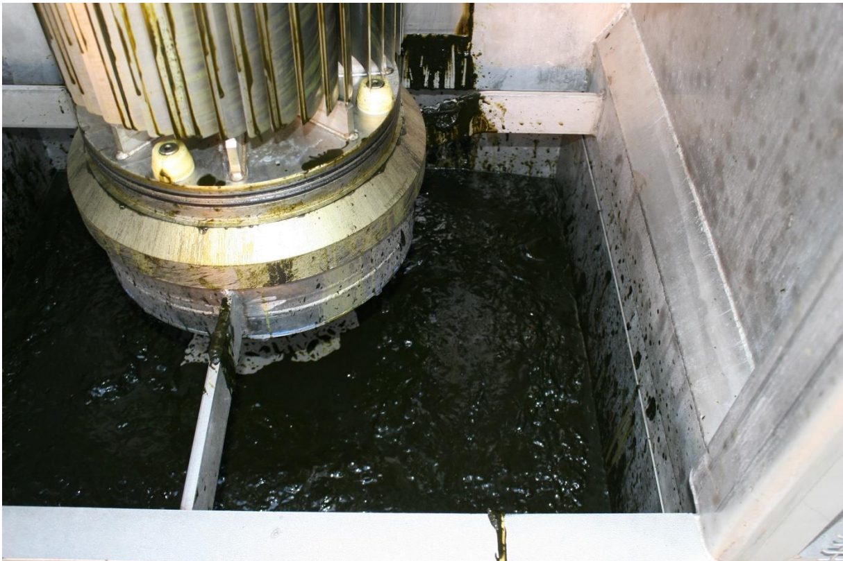
Picture 1: Photo of the concentrated Isochrysis galbana paste after centrifugation in an Evodos 25 dynamic settler
